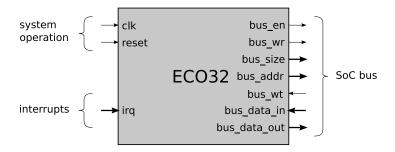
FIGURE 1. ECO32 Signal Interface
