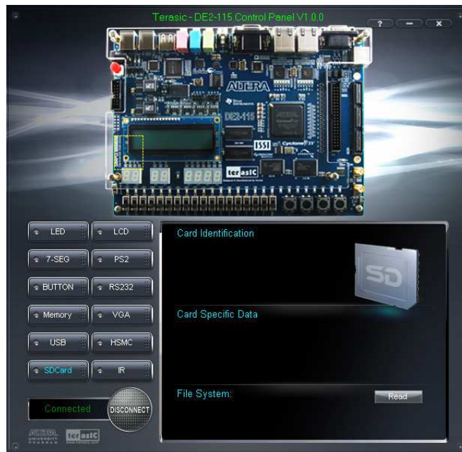
Figure 3-10 Reading the SD Card Identification and Specification
