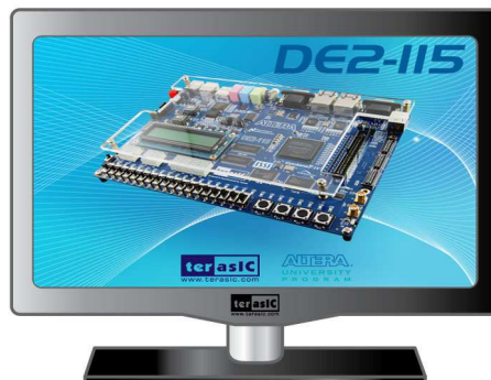
Figure 2-4 The default VGA output pattern
