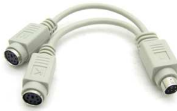
Figure 4-26 Y-Cable use for both Keyboard and Mouse
