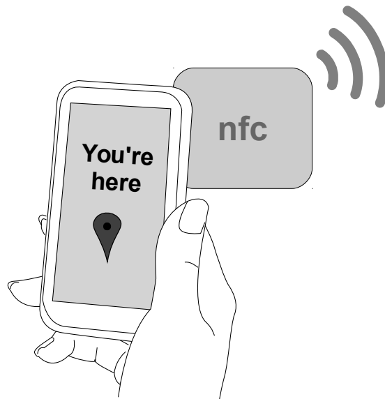
Figure 17.1.: Device Scanning a Passive NFC Tag
